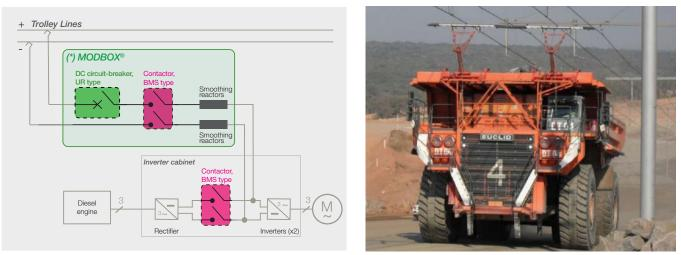
(\*) MODBOX<sup>®</sup> is an integrated system, compact and modular, for safe integration of high-voltage components on traction vehicles, running on AC or DC networks. Please refer to Sécheron brochure SG580044BEN.
