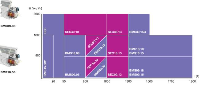
**Note!** Electro-pneumatic contactors type BPS are still in Sécheron's delivery program even if not represented on the above matrix.
